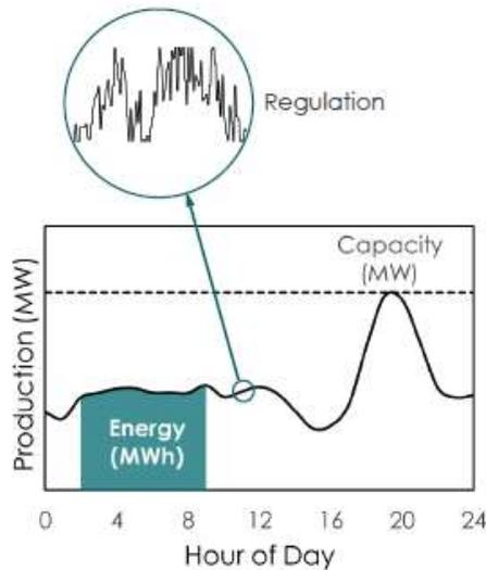
**Figure 2: Graphical Representation of Power System Planning Areas**
